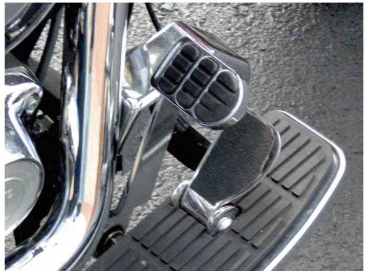
Wyatt’s floorboard throttle. Designed and built by Dr. Dave Clemons.
