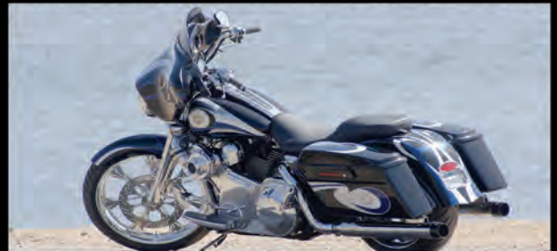
2007 Streetglide, 105 CI motor with ProCharger Blower, 171 rear wheel HP, FBI wide tire kit, DVD & NAV system, & Kenny Reynolds paint
